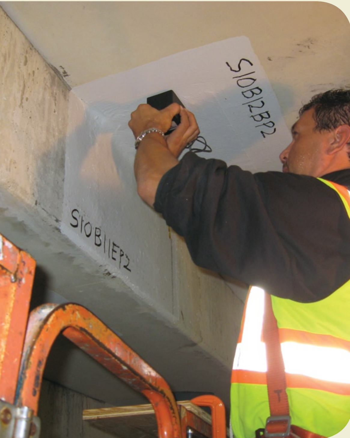
Composite patches at West Point's stadium are scanned using nondestructive acoustic wave guide sensors as part of a corrosion retrofit test project. Photo courtesy of Construction Engineer Research Laboratory, U.S. Army Engineer Research and Development Center. Page 18
